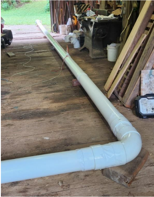
Figure (13): 6" Sweep 90-degree elbow
