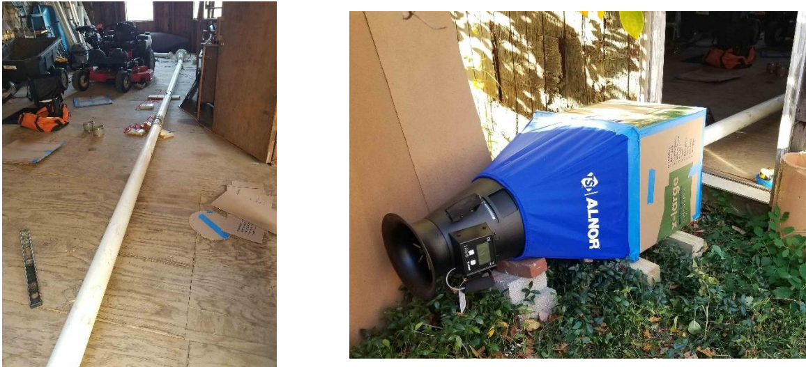
Figure (4): Alnor Balometer to Flow Grid Comparison
