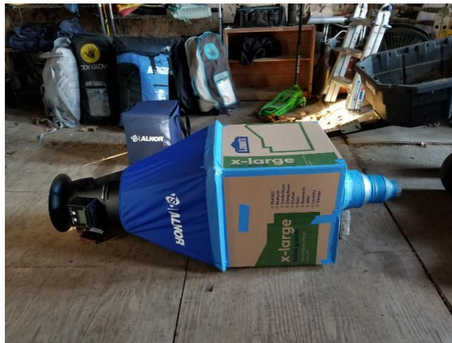
Figure (3): Smooth transition from Balometer to 4" PVC
