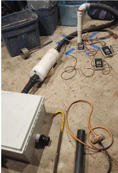
Figure (16): PFE test w/8 cavity test hole
