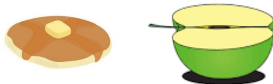
Figure (9): Sub-slab Area of Influence (AOI) is a hemisphere not a pancake
